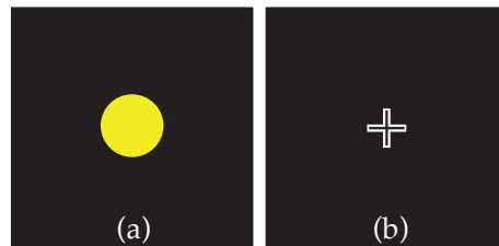
Figure 6.1: An illustration of the use of an area cursor in Sniper Pointing . (a) An area cursor can be used for coarse pointing. (b) The cross-hair is used for fine pointing.
